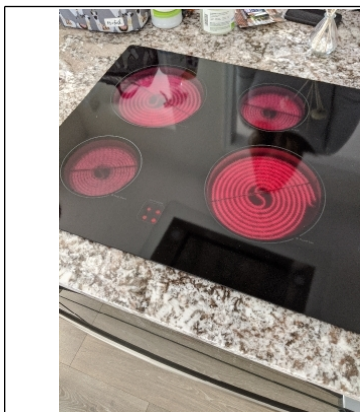
Operated a few seconds and tripped breaker
